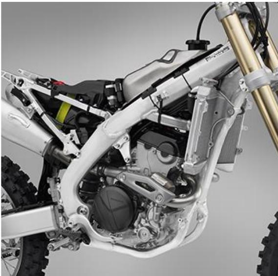
The 18YM CRF250R DOHC engine is a clean sheet design and has been built with the focus on top-end power for acceleration and drive, plus improved over-rev corner-to-corner.
