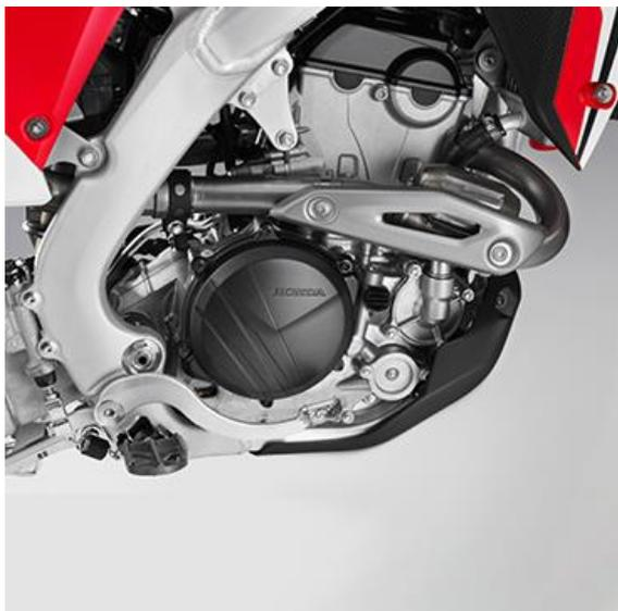
The 18YM CRF250R employs the same frame and suspension setup as the current CRF450R, with the same basic aims; connect the rider to the terrain with superlative feedback and gain rear wheel grip and drive through a rearward shift in weight bias, tied to a lower centre of gravity.
